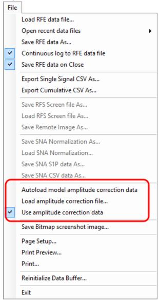
With this configuration, the noise floor will increase to adjust for actual reading. The sensitivity is also adjusted to that of the antenna, and therefore direct amplitude readings makes signal trace power measurement a breeze.
