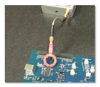
Compared with other near field antennas, RFEAH are smaller and lighter, exactly what fits best when space is constrained in a PCB.
