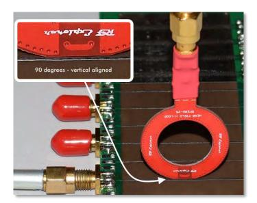
The H-Loop antenna works basically as an inductive coil, capturing magnetic flux. Therefore, it should be oriented in such a way the maximum magnetic field is captured.
