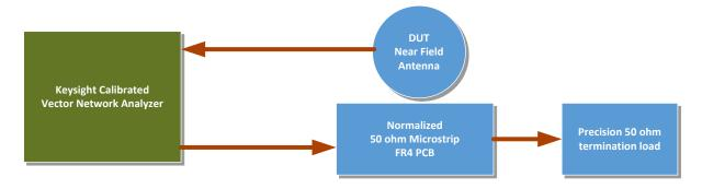
The antenna must be vertical 90 degrees against PCB signal trace, at 0mm distance, parallel horizontal orientation to signal trace for maximum sensitivity of the magnetic flux, as depicted below.
