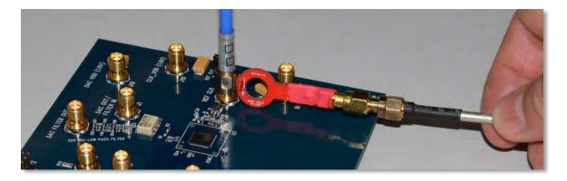
There are three different magnetic antenna options: As the antenna diameter gets shorter, the spatial resolution increases at the cost of some sensitivity loss at low frequencies, but best response at high frequencies; you should select RFEAH-25 for best sensitivity with connectors, large ICs and isolated signal traces, whereas RFEAH-5 works best for very narrow selective work in a populated PCB with close-by signal traces. RFEAH-15 is a good in-between compromise.
