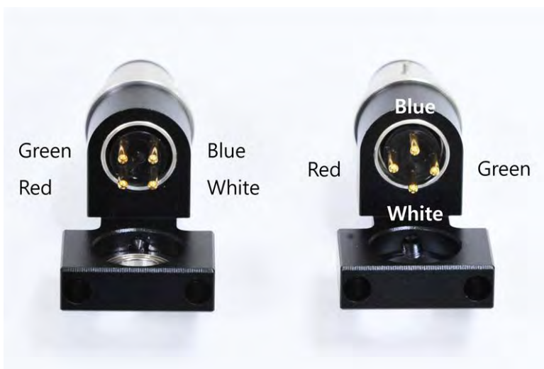
Lead wire connection
